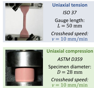
Fig. 6. Uniaxial tensile and compression tests were performed on the silicone specimens
