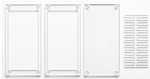
Fig. 4. Parts of the laser-cut acrylic mould for the rectangular soft actuator
