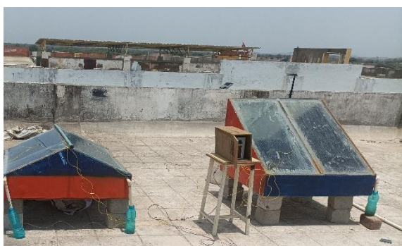
Fig. 4. Single and double slope solar still experiment setup (Location Bhopal)
